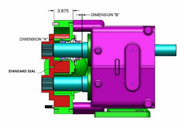
2) See table below to determine proper seal setting for inner and outer seal. Due to the seal setting flexibility, the seal setting is calculated in .015" increments.
